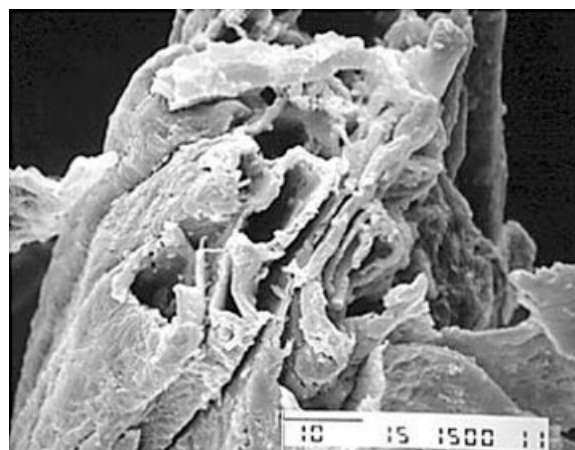
Figure 1 Scanning electron microscopy image of SCB fibers.
